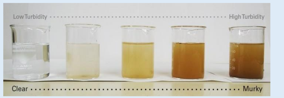
Figure 13. Turbidity samples; low turbidity measured in nephelometric turbidity units (NTU) to high NTU from left to right.
